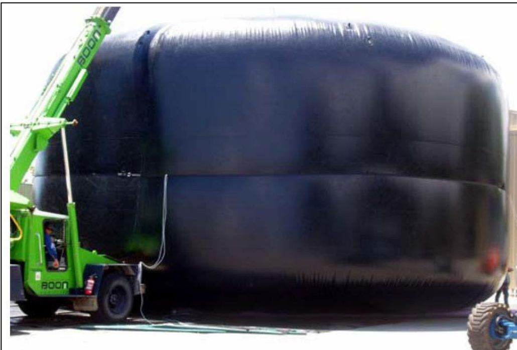
Figure 32: Inflatable shaft seal
