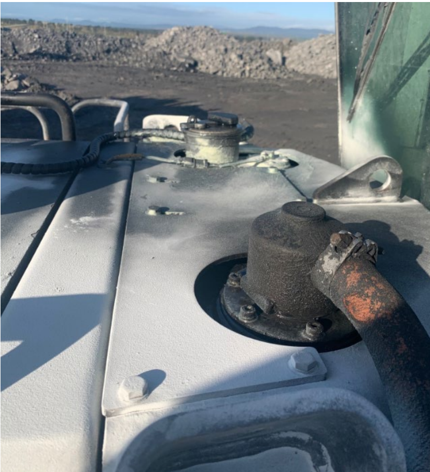
Figure 2 - Level control vent and filler cap
