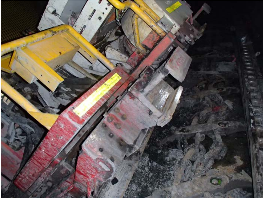
Figure 1 Rapid face bolter tipped 45° towards the face
