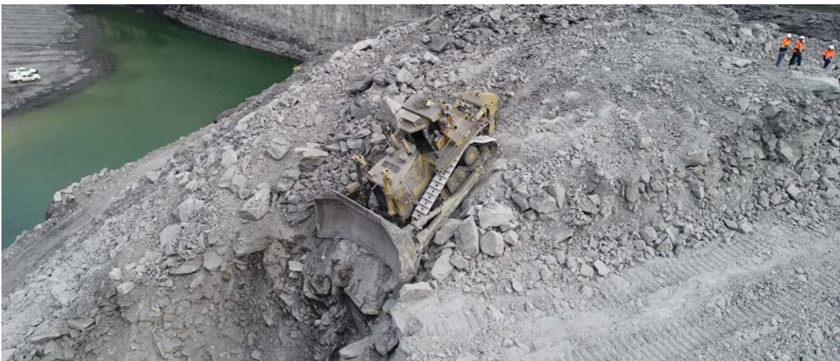
Figure 1 A near miss over a drop off at a coal mine in the Hunter Valley
