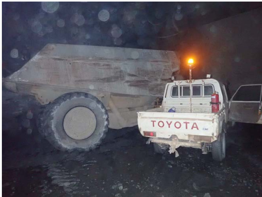
Figure 1: Haul truck hits light vehicle (IncNot0033382). Photo by NSW Resources Regulator
