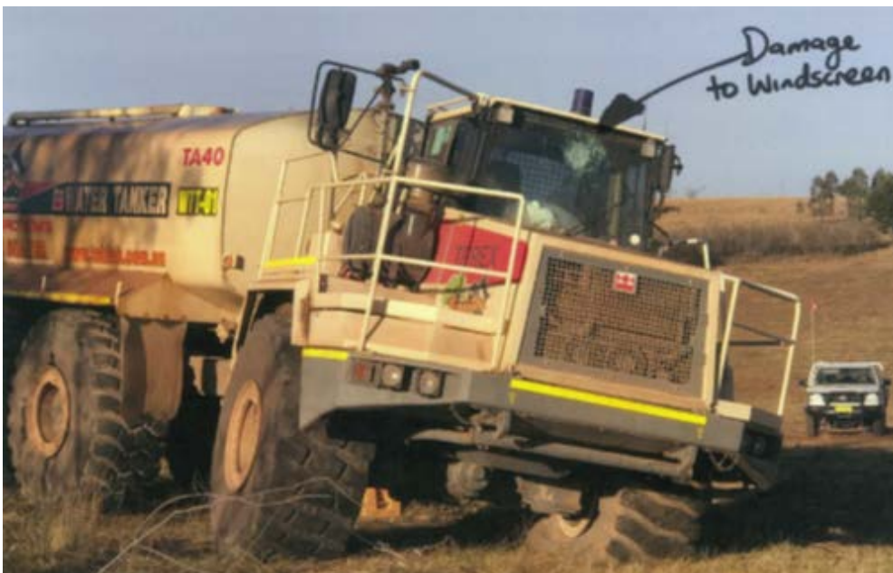
Figure 3: A piece of wood ejected from a mulching machine struck the windscreen of a water cart. (SinNot-2017/01683)
