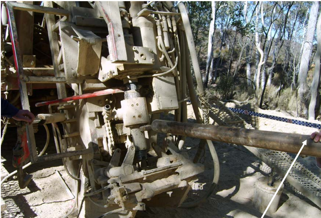
Drill Rig with Drill Rod Being Used as a Lever
