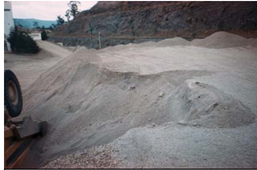
Top of stockpile – Note: bunding not sufficient to stop truck rolling
