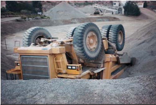
Truck on back where front-end loader had been removing material
