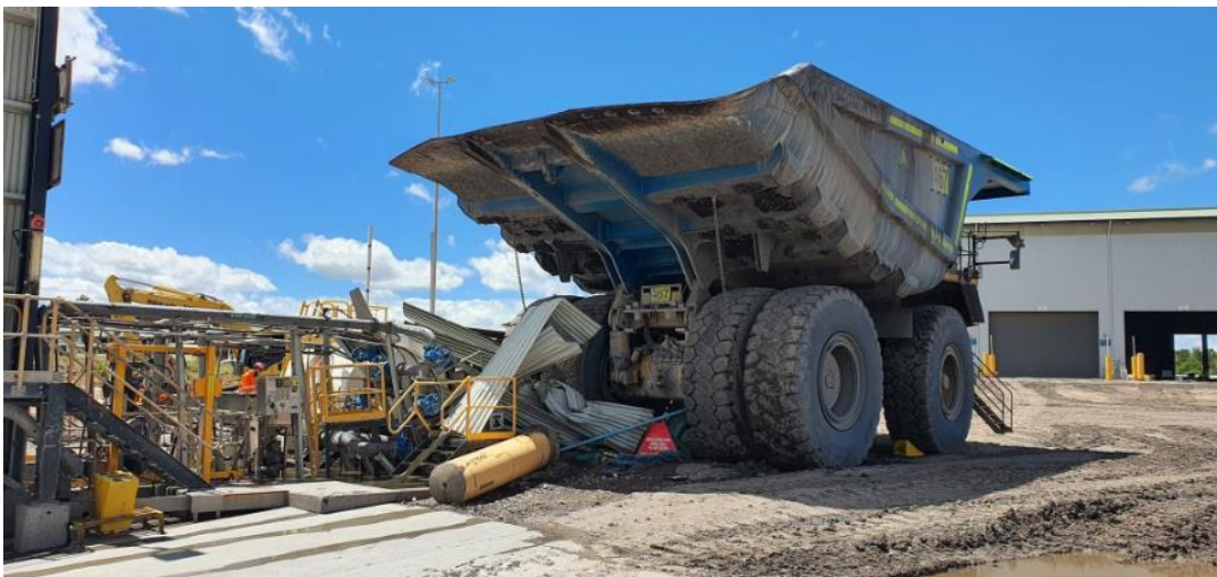
Figure 1 Truck collision with wash bay pump
