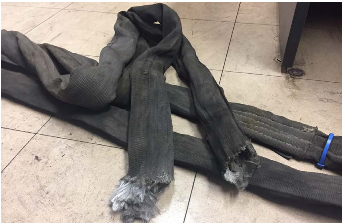
Figure 2: The failed sling
