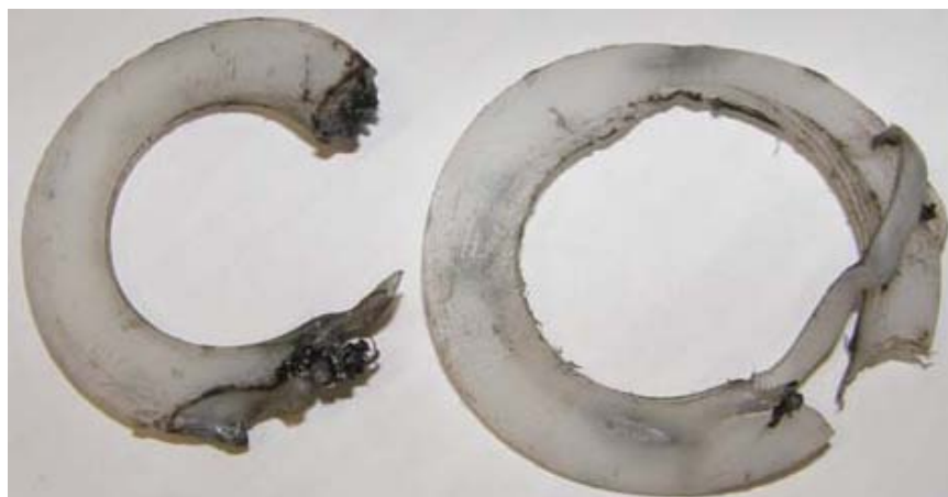
Photo: A partially melted washer (left) and an ignited washer (right).
