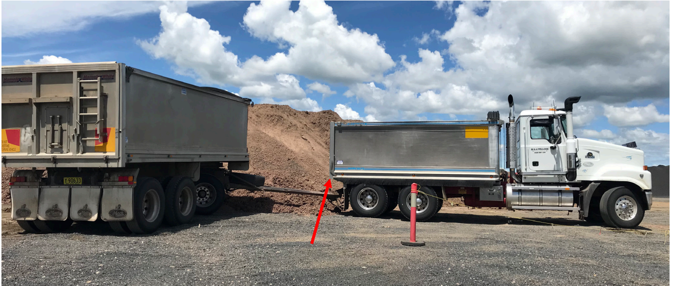
Figure 1 The red arrow shows where the truck driver's head was when it was hit. Note: the tray was in a raised position when the incident occurred.
