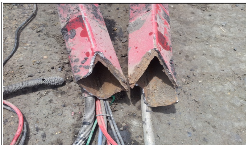
Figure One – Failed drawbar on dog trailer
