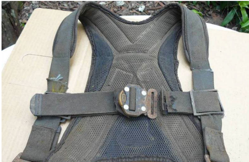
Figure 18: The condition of the rigger's harness (taken post incident) laid out in an as-worn configuration. Note some of the visible damage to the harness was sustained as a result of the recovery of the injured mine worker. 30
