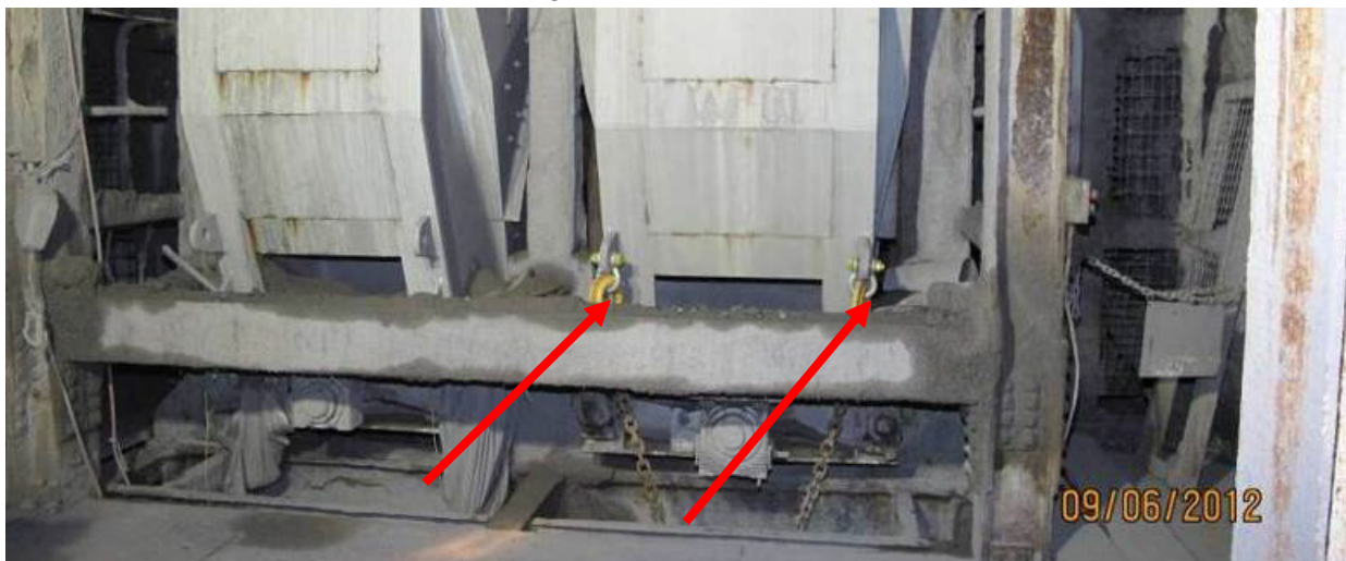
Figure 6: Two yellow chain hooks attached to the lugs on the weigh flask.
