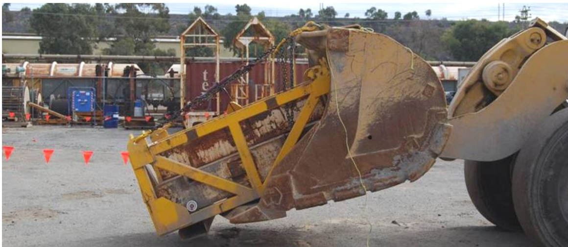
Figure 12: The angle of the bucket required for the weight basket to slide from the bucket. Note the weight basket was tethered by a chain for the purpose of the test. 20
