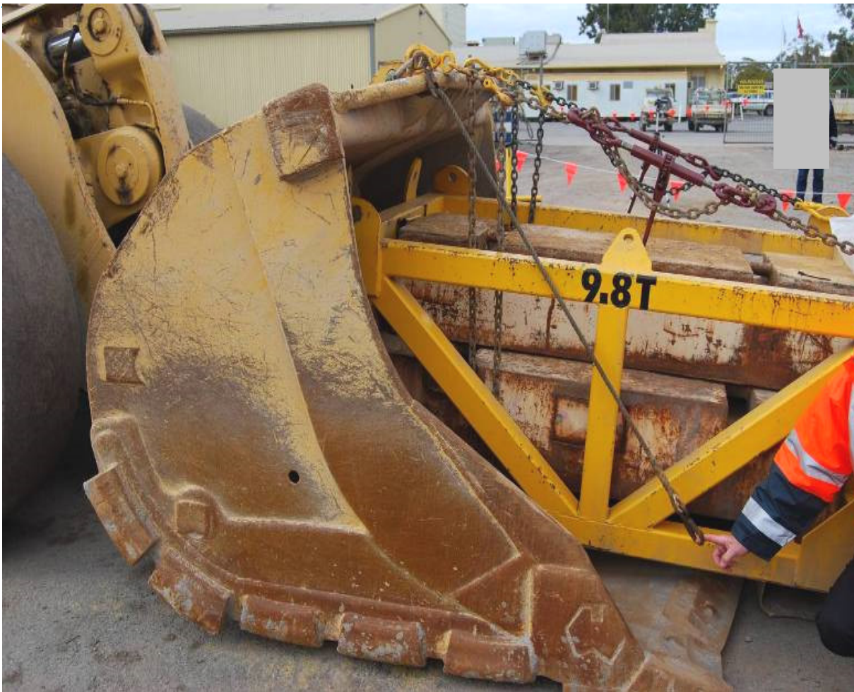
Figure 22: The distance that a 2 metre lanyard would extended laterally and vertically towards the tip edge of the bucket when the lanyard was back hooked to the top of the bucket. It was observed that the lanyard end would not reach to the front tip edge of the bucket. 33
