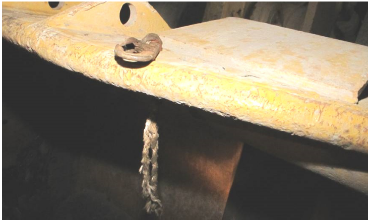
Figure 9: The rigger's rope lanyard end as found reeved onto a hole in the loader bucket. 18
