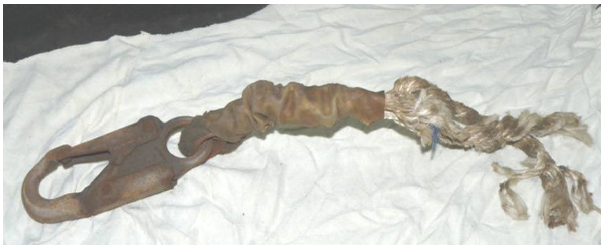
Figure 17: Remnant of the injured rigger's fall arrest lanyard as found on the loader bucket. Note the remaining components of the failed lanyard have not been recovered from the base of the shaft. 1
