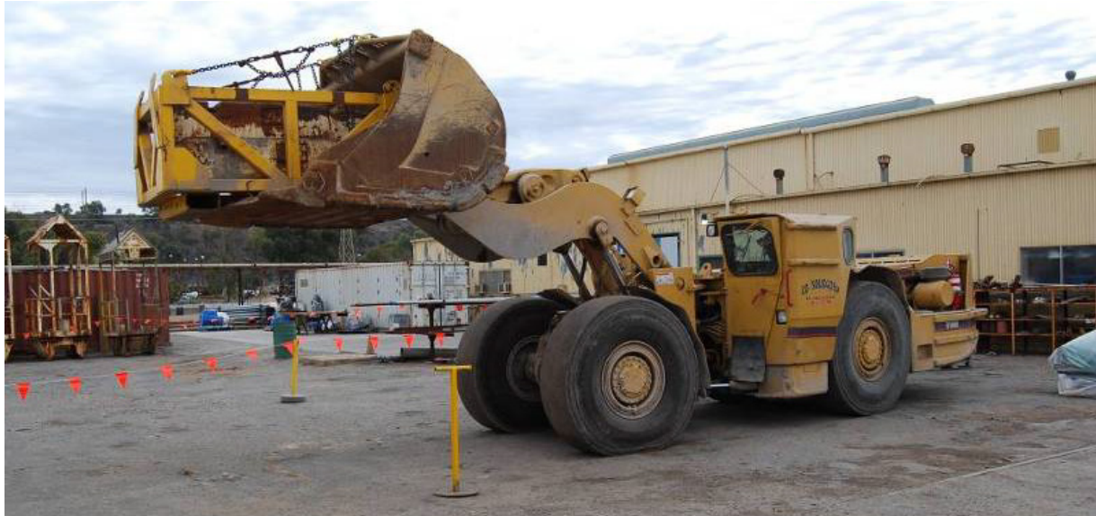
Figure 13: The loader bucket in a raised position on 28 June 2012. The yellow marker post in front of the loader represents the height of the shaft gate. 21
