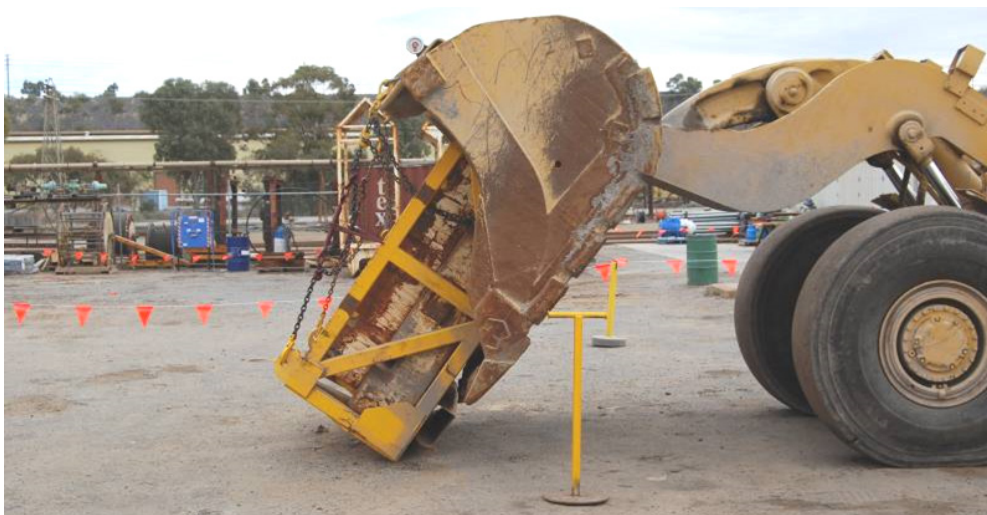
Figure 14: Observation made on 28 June 2012 showing the final resting position of tethered basket and bucket following the loss of control of the load by the operator during the operation of the load at full elevation. 22
