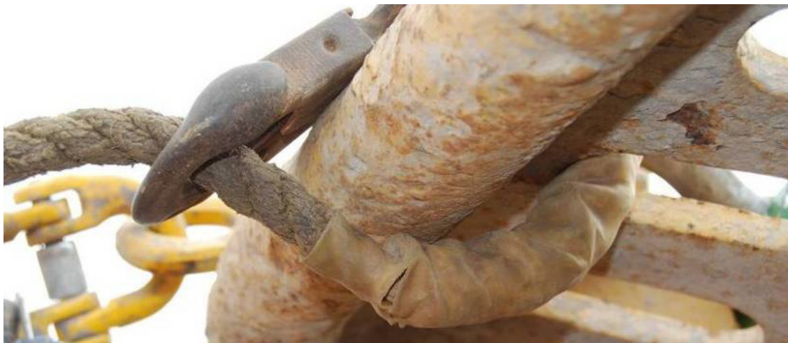
Figure 19: A simulation of the lanyard reeving method back hooked around the sharp edge hole in the loader bucket. The simulation used by the assistant mine worker's rope lanyard, which was similar to the lanyard that the rigger used. 31
