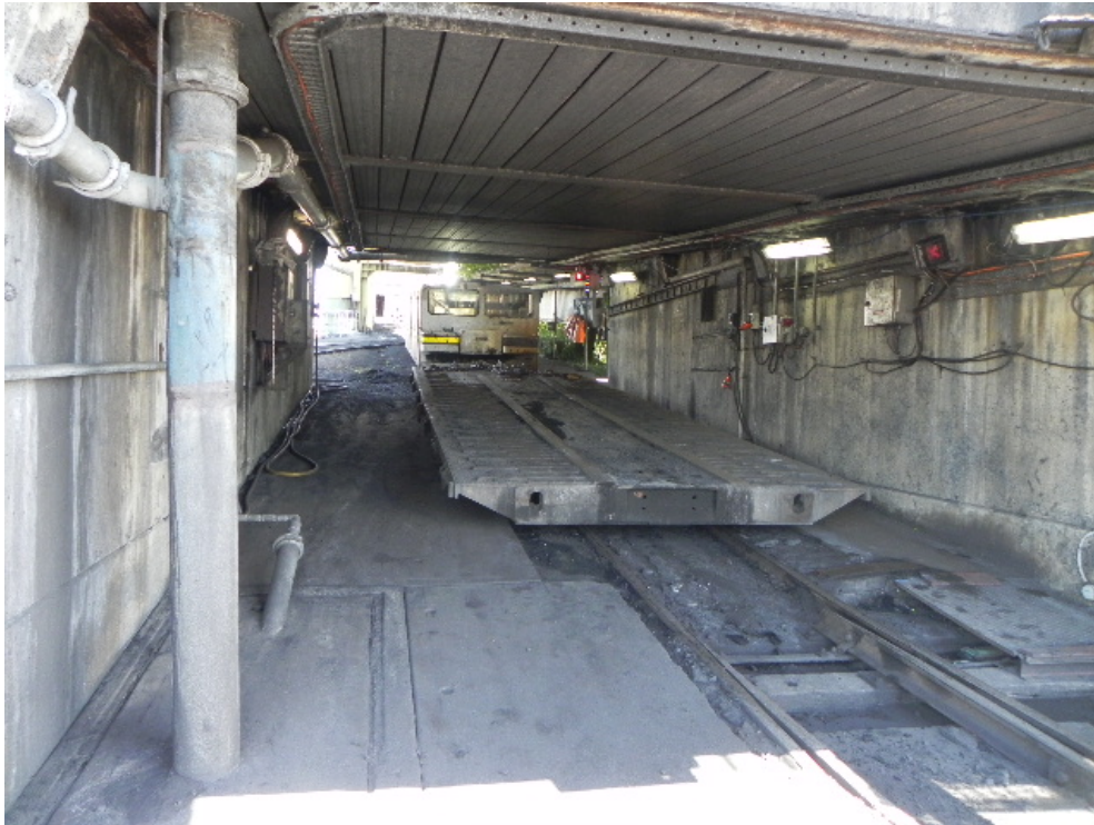
Figure 16 Example of drift haulage control car and flat top (materials transport system)
