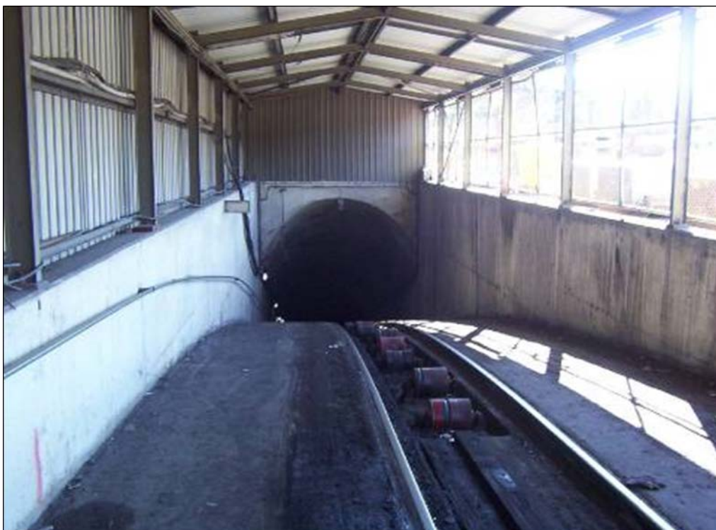
Figure 12 Drift rope haulage crest rollers
