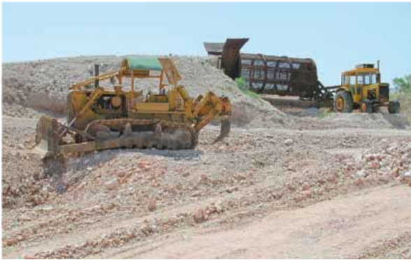
Figure 96 - A trommel used for reducing the amount of opal dirt to be processed
