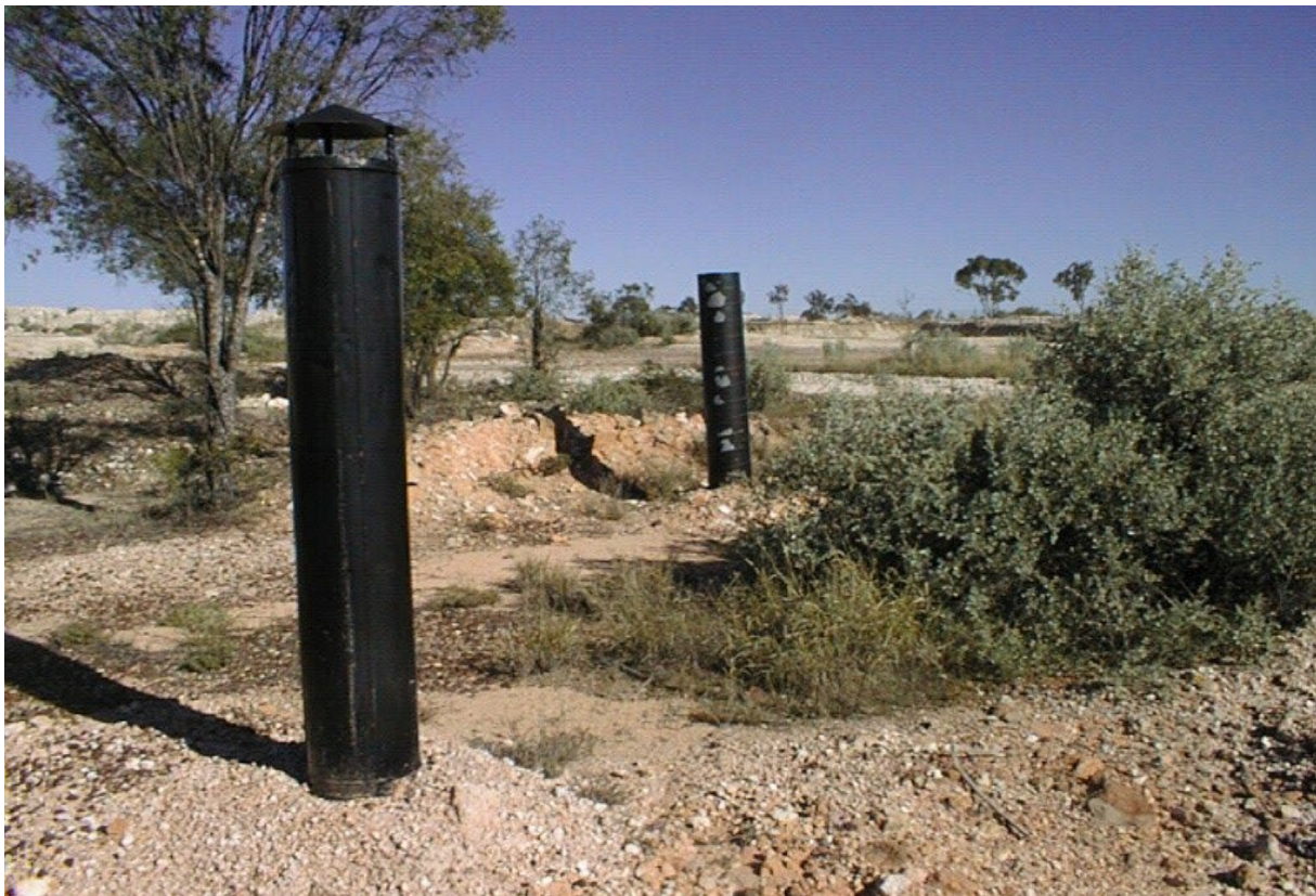
Figure 84 - Black pipe over an auger hole used to help natural ventilation
