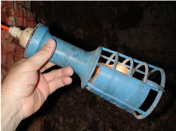
Figure 146 - Protected light fitting, household globe.
