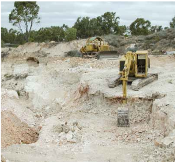
Figure 94 - Removing the opal level using a 15-tonne excavator
