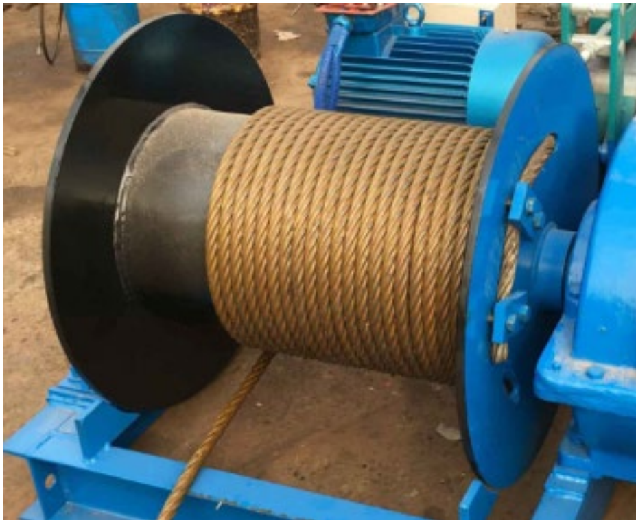
Figure 118 - Rope anchorage on drum
