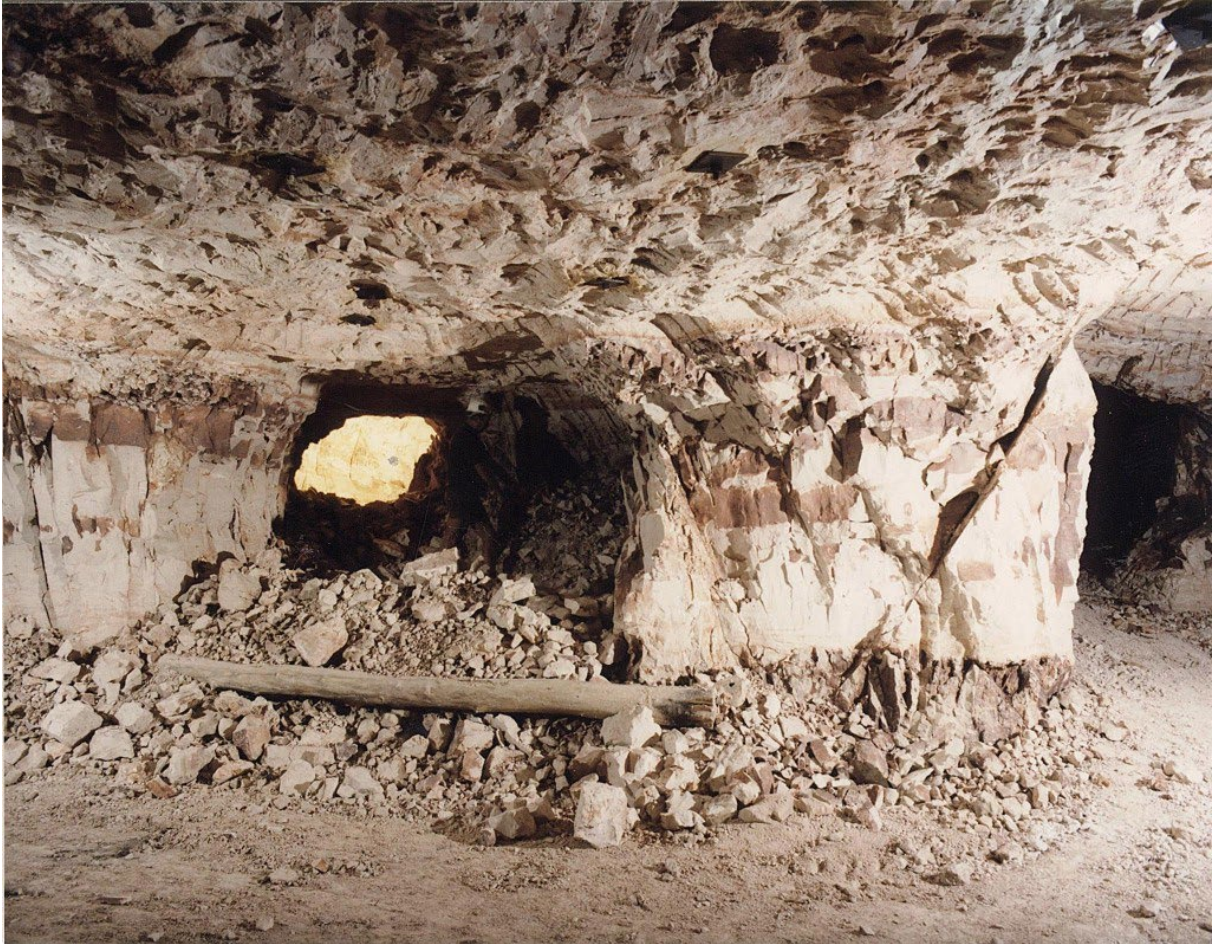
Figure 74 - Room and pillar mining
