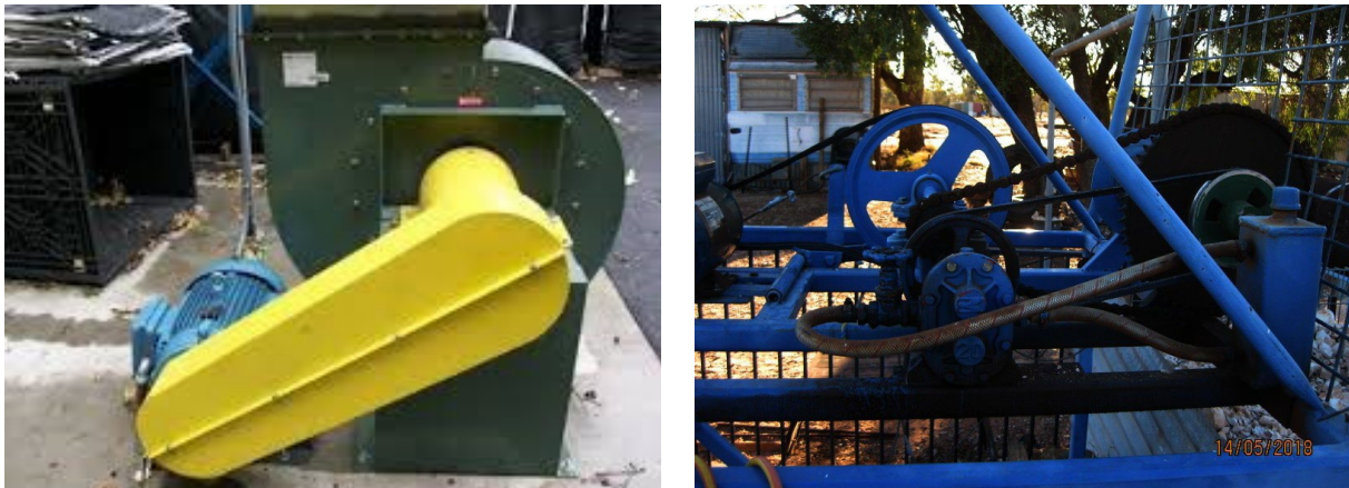
Figure 105 - Other examples of good (left) and bad (right) guarding
