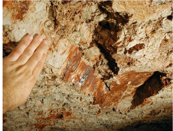
Figure 33 - Exposed fault plane in a mine roof
