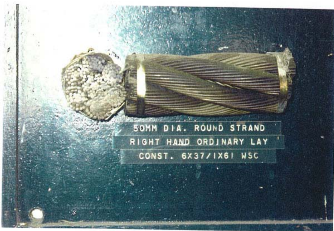
Typical Winding Ropes Fig 2.4
