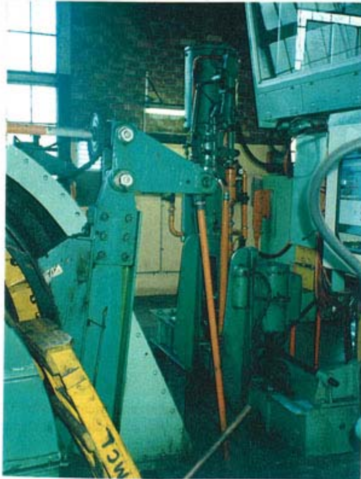
Whitmore overwinding mechanism associated with post brake
