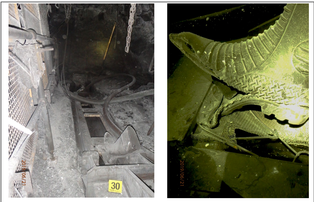
Figure 11. Gumboot and mesh entangled in conveyor flight bar
