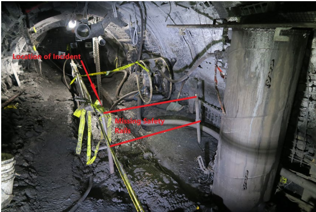
Figure 15. Emergency lanyard control box with missing lanyard
