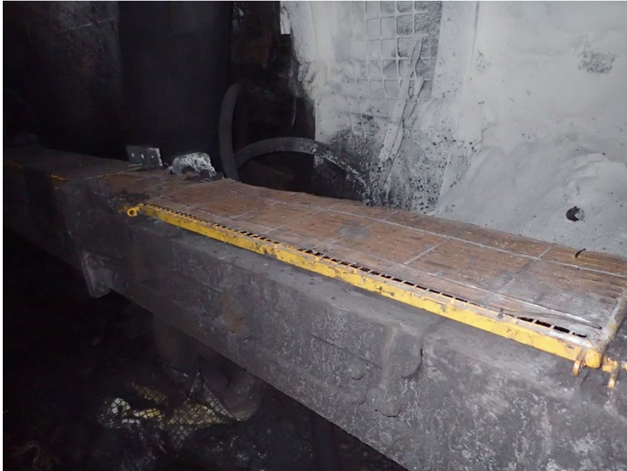
Figure 13. Tech mesh fitted to the top of the yellow guard on the scraper conveyor
