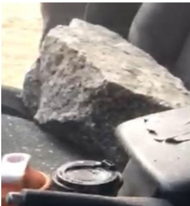
Figure 1 Flyrock on driver's seat of shotfirer's utility
