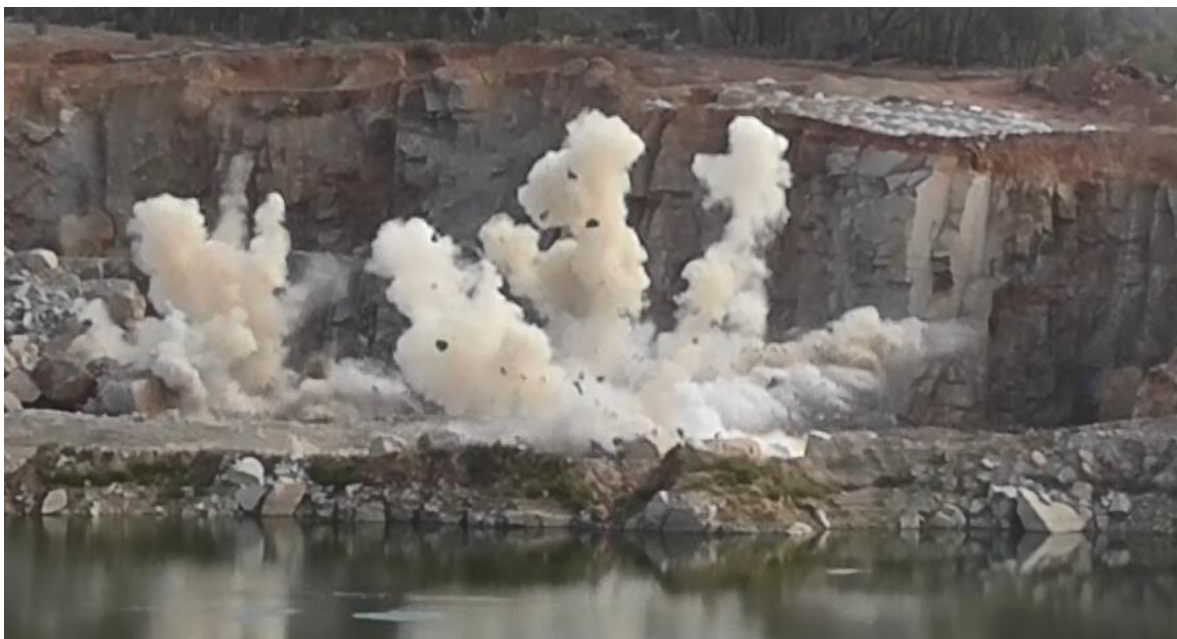
Figure 7 - Flyrock produced by toe blast
