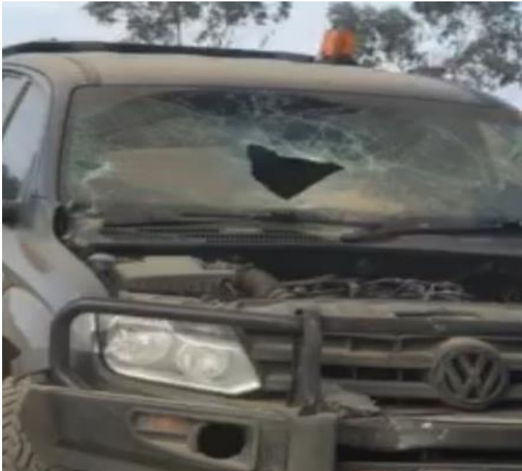
Figure 10 - Damage to shotfirer's utility
