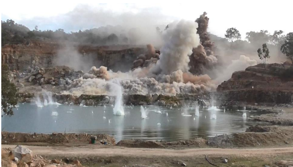
Figure 9 - Flyrock landing in dam in front of firing location
