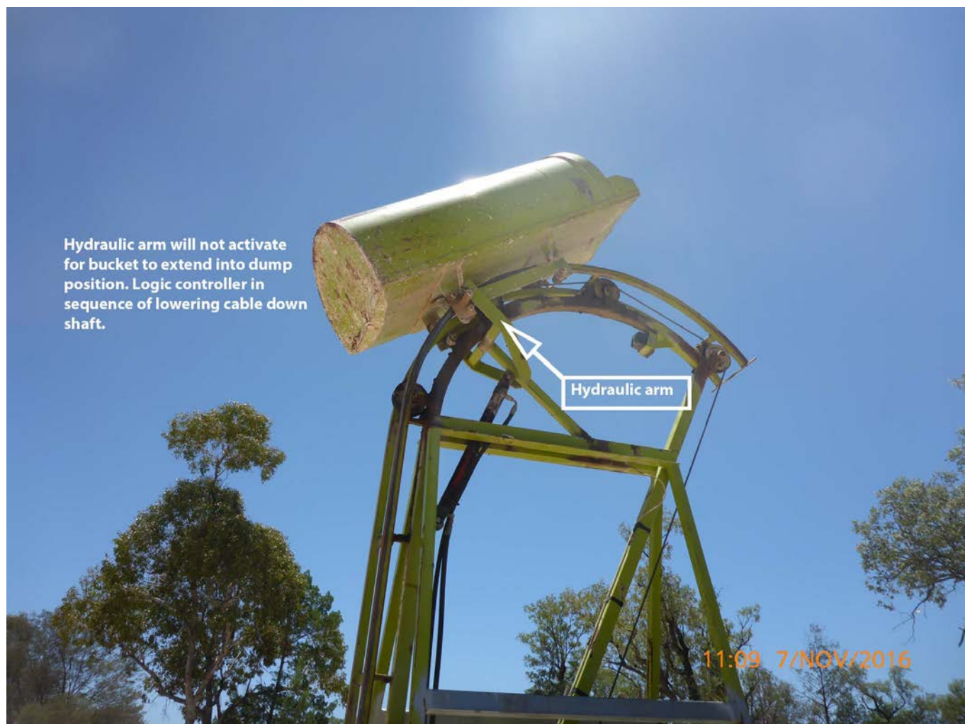
Figure 25: The bucket unable to fully engage into the tip position.
