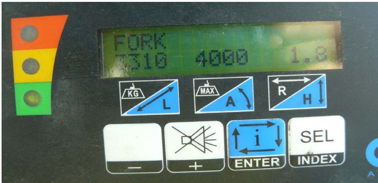
Figure 7: Operating panel inside the telehandler showing the three indicator lights that operate when the machine is lifting a load.
