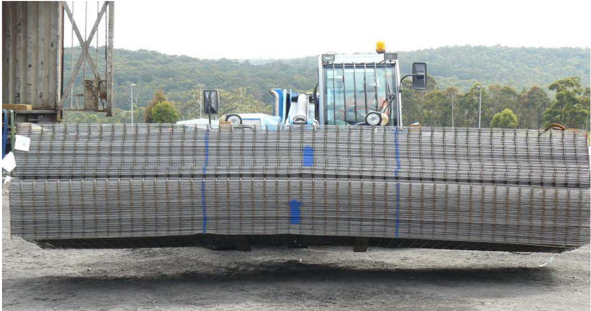
Figure 3: Telehandler carrying two bundles of mesh.
