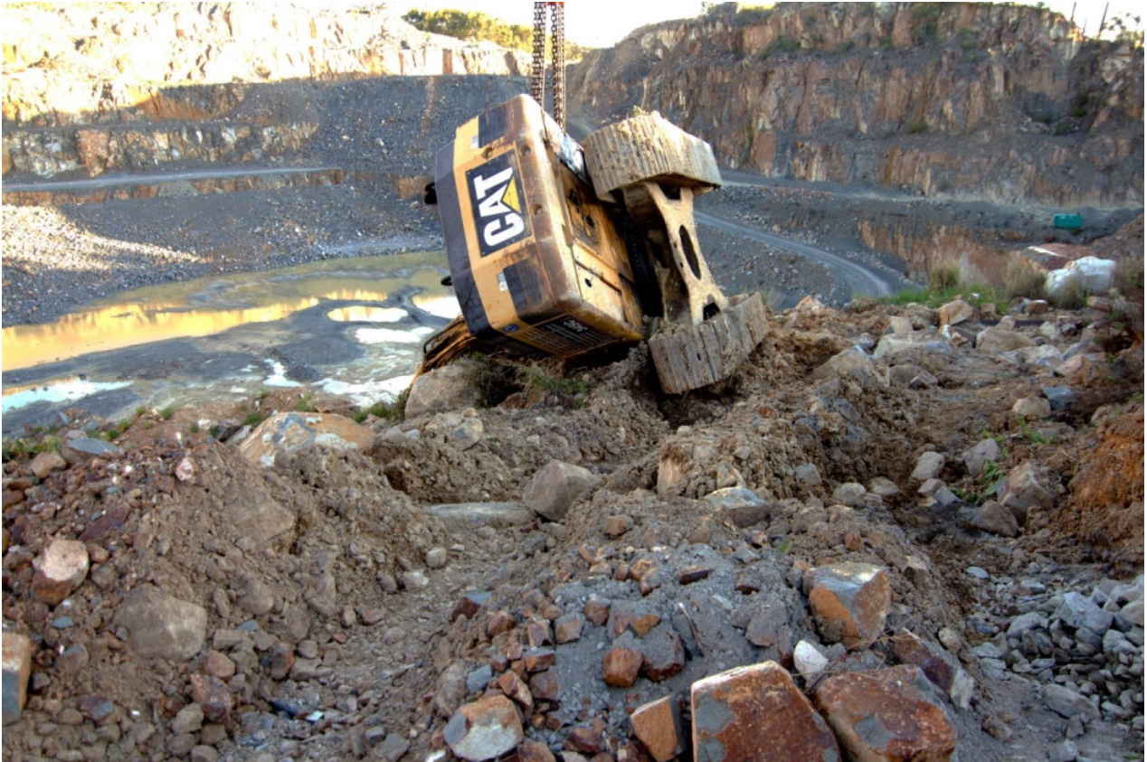
Image 4: Orientation of superstructure to the track frame on excavator - Photograph by Investigation Unit
