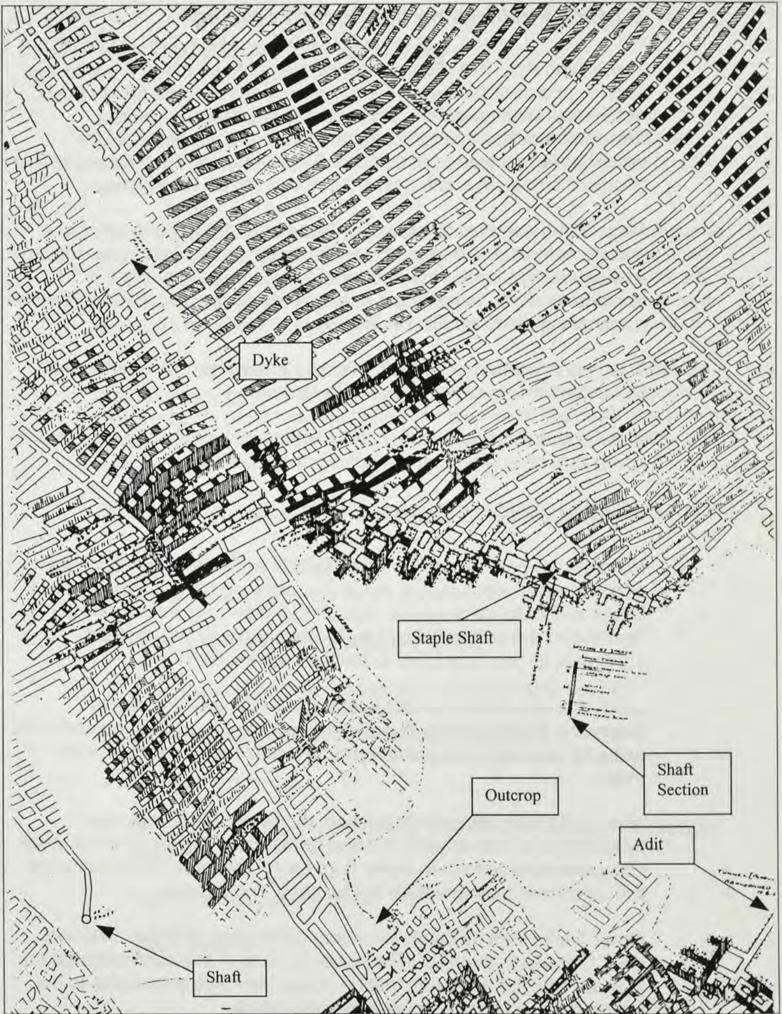
Example 3 Points to note Shafts, Geology Sections
