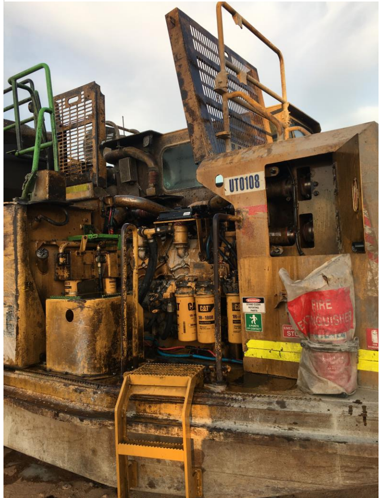
Figure 1: Engine bay covered in hydraulic oil
