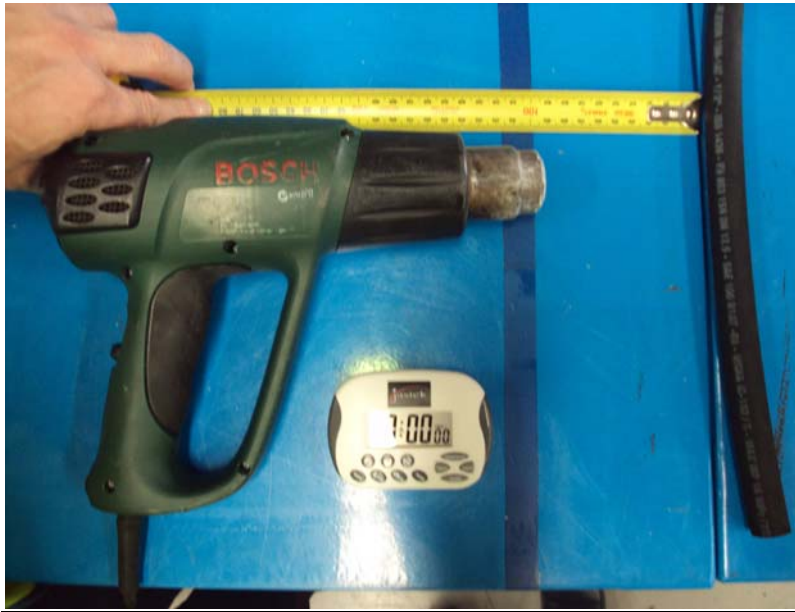
Image 2 – Showing test set up 200mm distance
