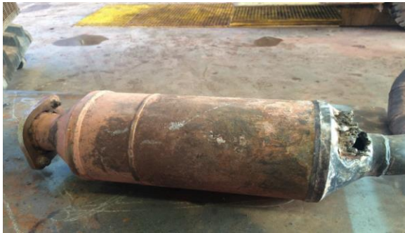
Fig. 1 Toyota Landcruiser Partial Flow DEF subject to catastrophic uncontrolled regeneration.
