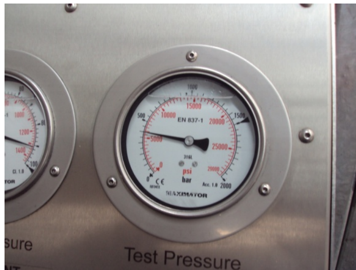
Image 4 – Showing calibrated test gauge reading
