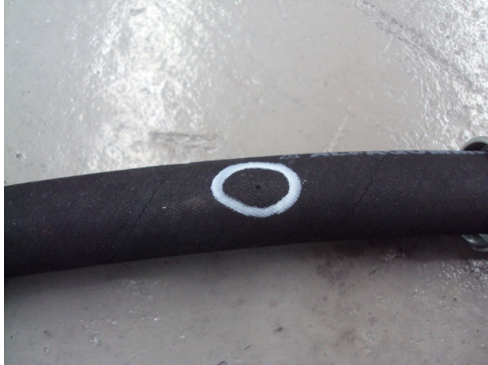
Image 2 – Showing pin hole preparation on test sample
