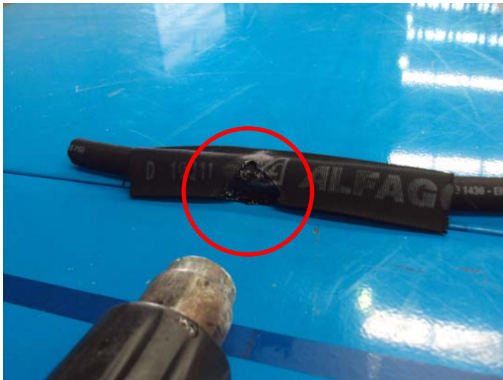
Image 3 – Showing sleeve sample type 1 melting
