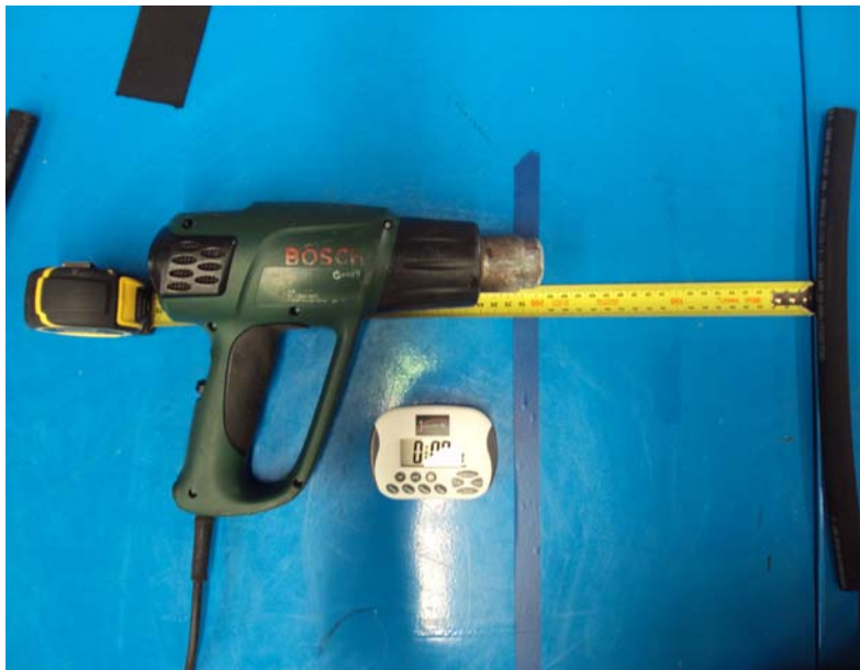
Image 2 – Showing test set up 200mm distance
