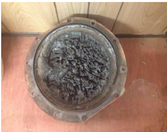
Fig. 3 Melted core of truck DEF after uncontrolled regeneration
