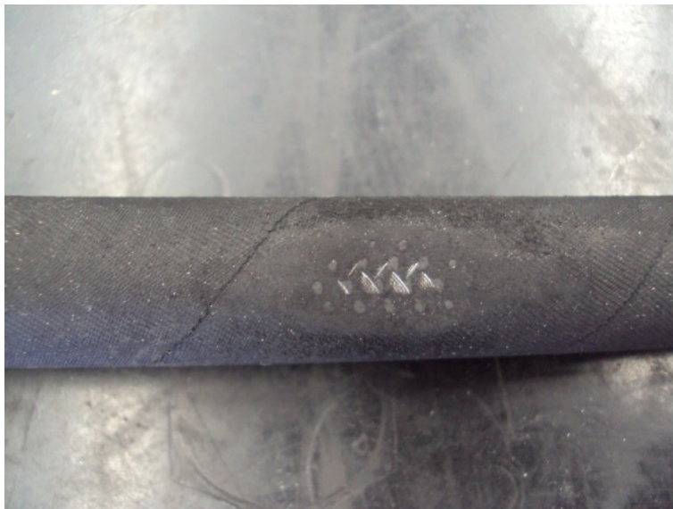
Image 3 – Showing wear damage preparation on test sample
