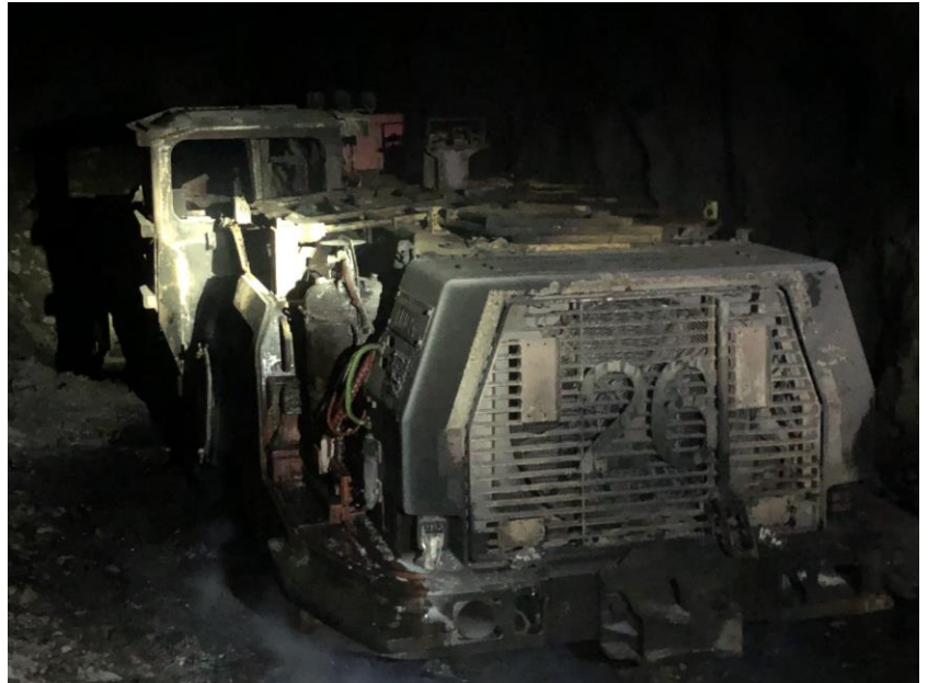
Figure 2a and 2b. Broken wire to brake solenoid causes fire to loader being operated under tele-remote conditions
