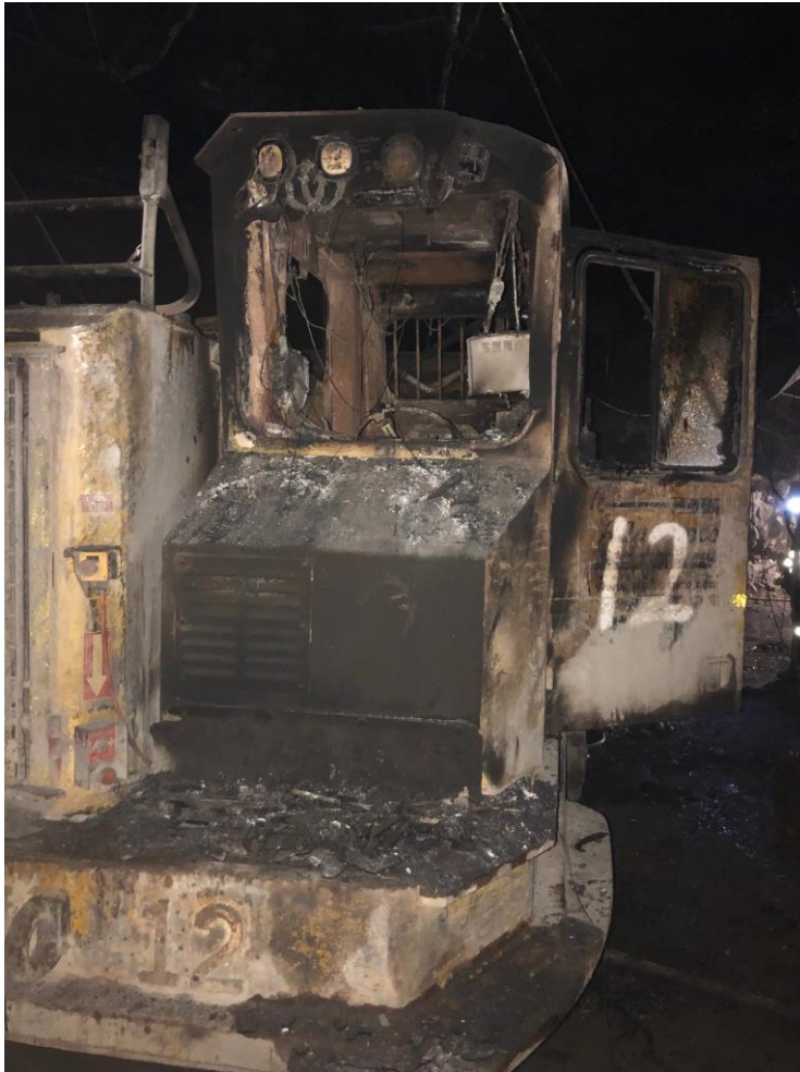
Figure 1. Short to earth in power supply to starter motor causes fire on haul truck
