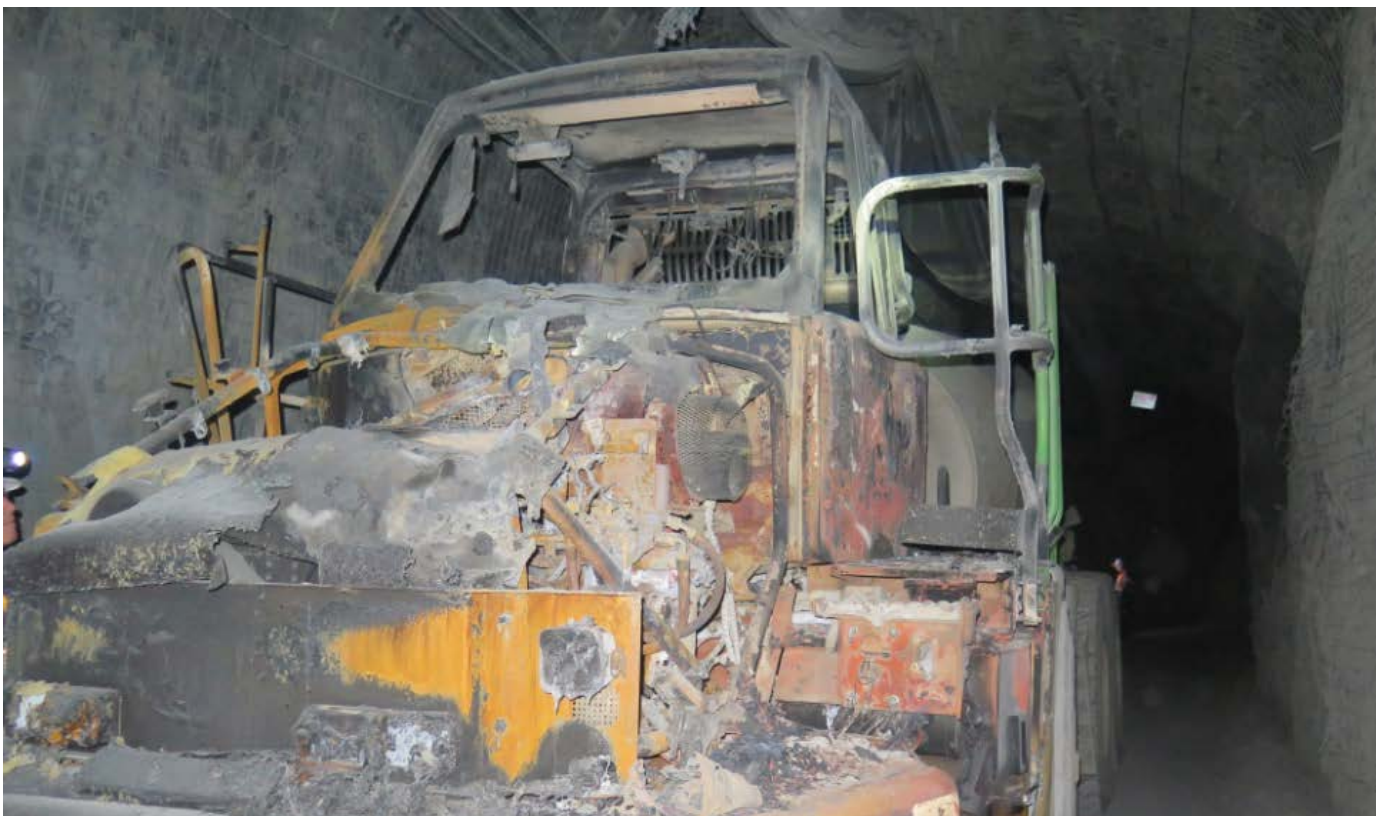
Figure 1 One of the nine underground fires fuelled by diesel and non-metallic materials
