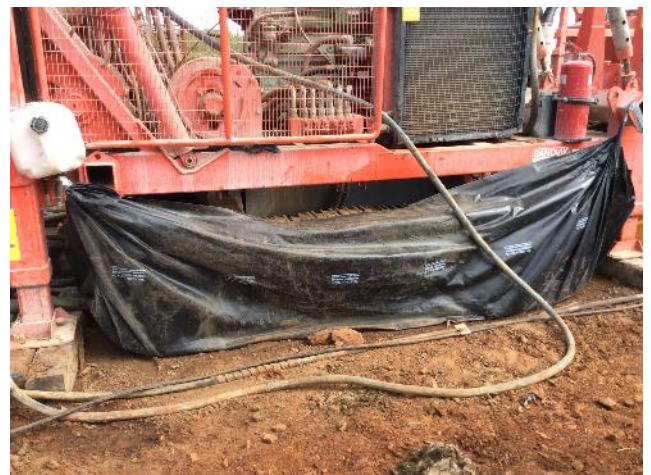
Figure 4 Rig nappy under the drill rig
