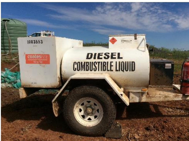
Figure 2 Diesel stored in a self-bunded tanker trailer
