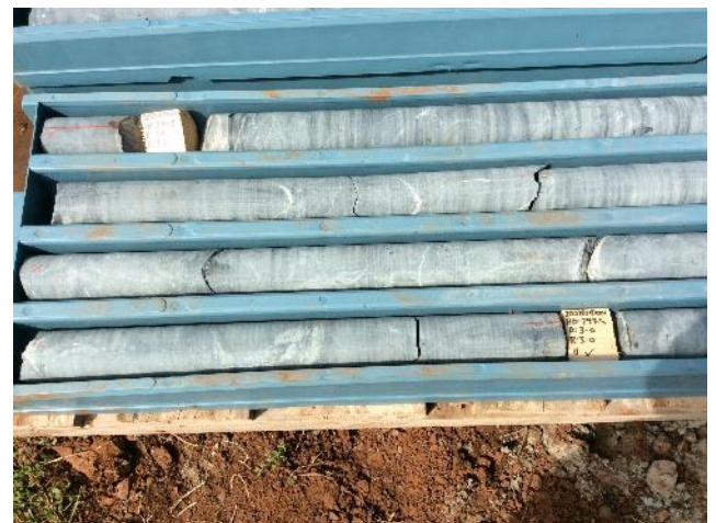
Figure 13 Example of core storage
