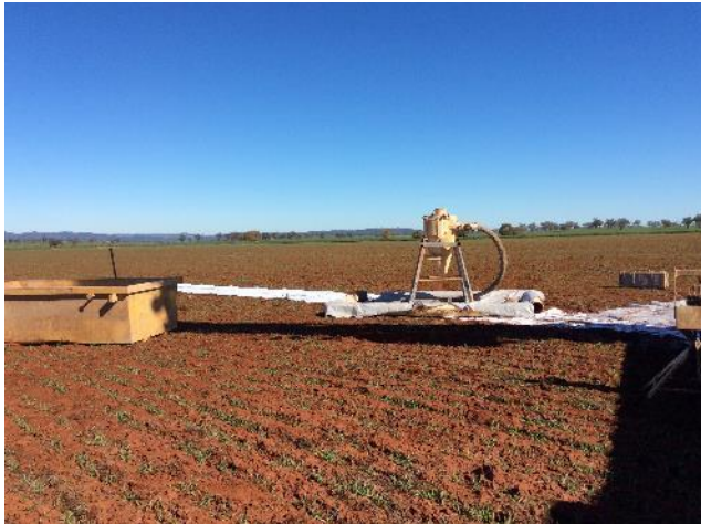
Figure 2 Return water system from drill rig at site 20LIRC010
