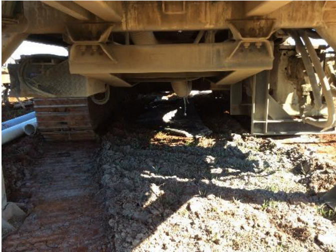
Figure 1 Rig nappy in place under the drilling rig
