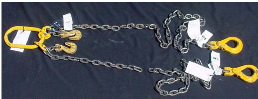
General view of the two leg chain set. Both chain legs were broken.
