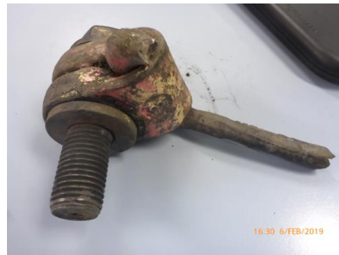
Figure 4: The failed incident 8t Rud link (source NSW Resources Regulator)
