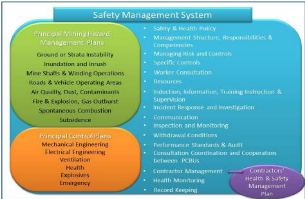
Figure 4. The elements of a safety management system (from Safety Management Systems in Mines COP , p.6).
