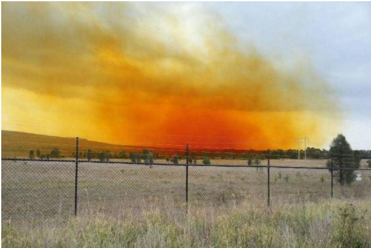
Figure 1. Orange blast fume plume over Muswellbrook after a blast at BHP's Mt Arthur Coal Mine (from Lamcraft, 2014).
