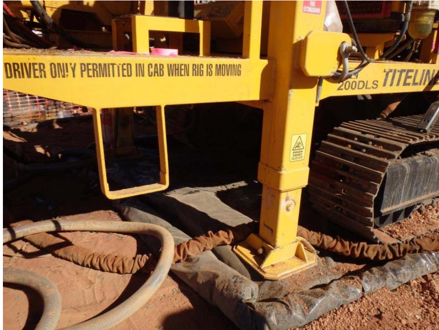
Figure 7 Spill control matting under the drill rig
