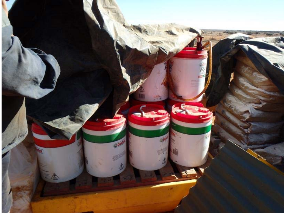
Figure 5 Oil drums stored on a banded pallet covered with a tarpaulin
