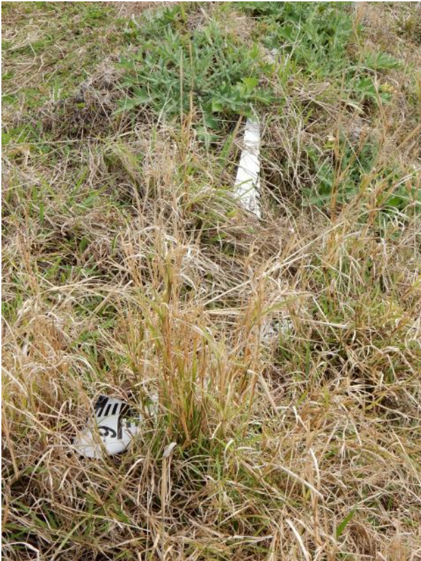
Photo 9 – Damaged gauge marker board on a major water storage at one site
