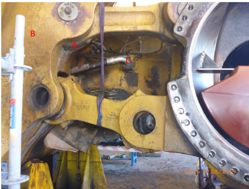
Figure 1 Left hand side lower link and pin assembly (A), front pin location (B), rear pin location (C)
