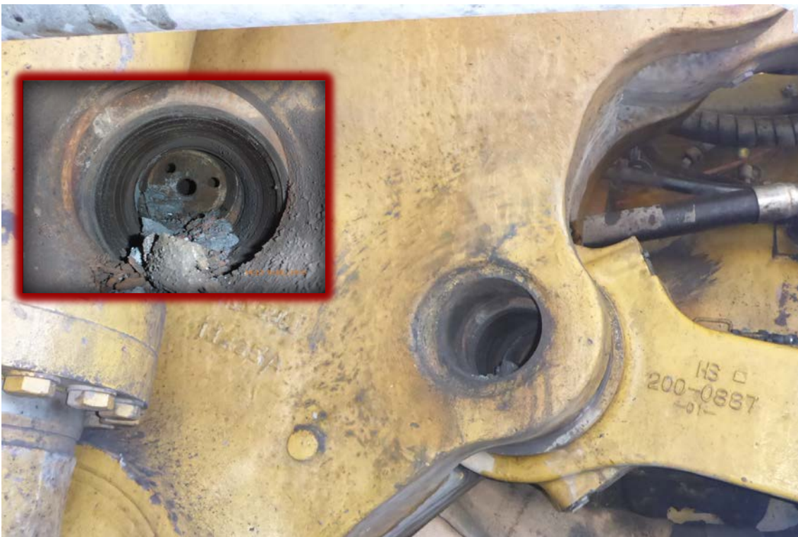
Figure 5 Pin bore with slag remnants
