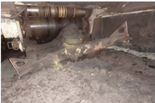
Figure 1 - Failed hitch point on DMU.
