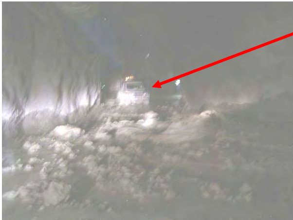
Photograph of the light vehicle bogged in the inrush material below VR5B shaft.
