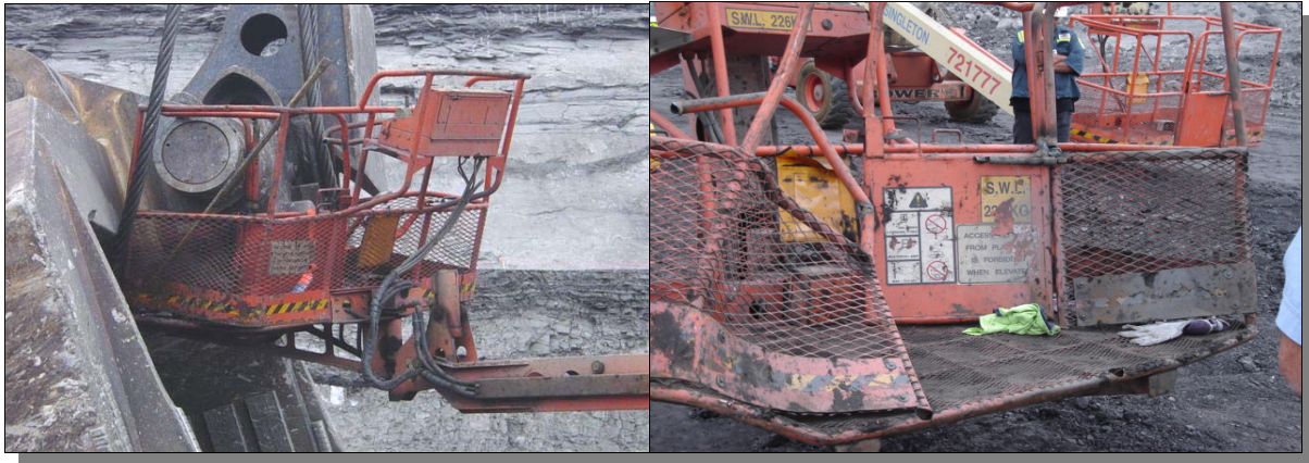
Man-basket, hoist ropes and equalizer
