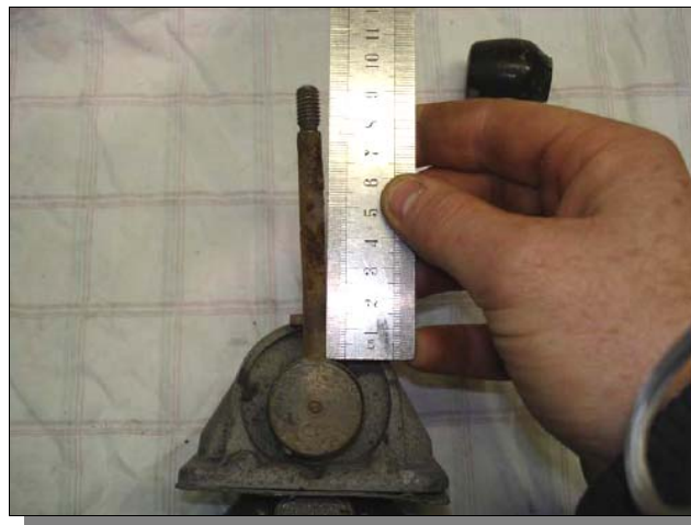
The bent centre shaft of the drive controller
