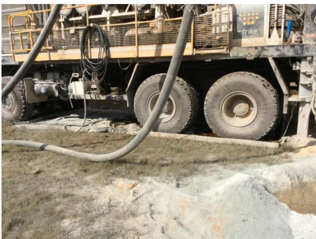
Figure 4 Rig nappy in place under Strike Drilling rig
