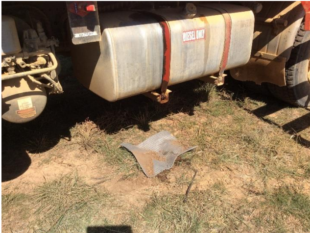
Figure 7 Spill matting in place to catch drips from Durock air core rig
