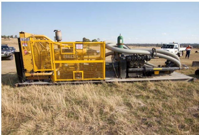
Figure 15. A Silver City Drilling Triplex mud pump on site at Ashton Coal Operations premises.
