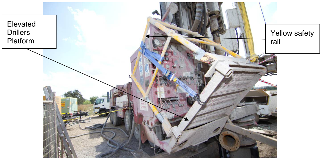
Figure 9. The driller's platform in a simulation designed to show the trajectory that was possible during the incident.
