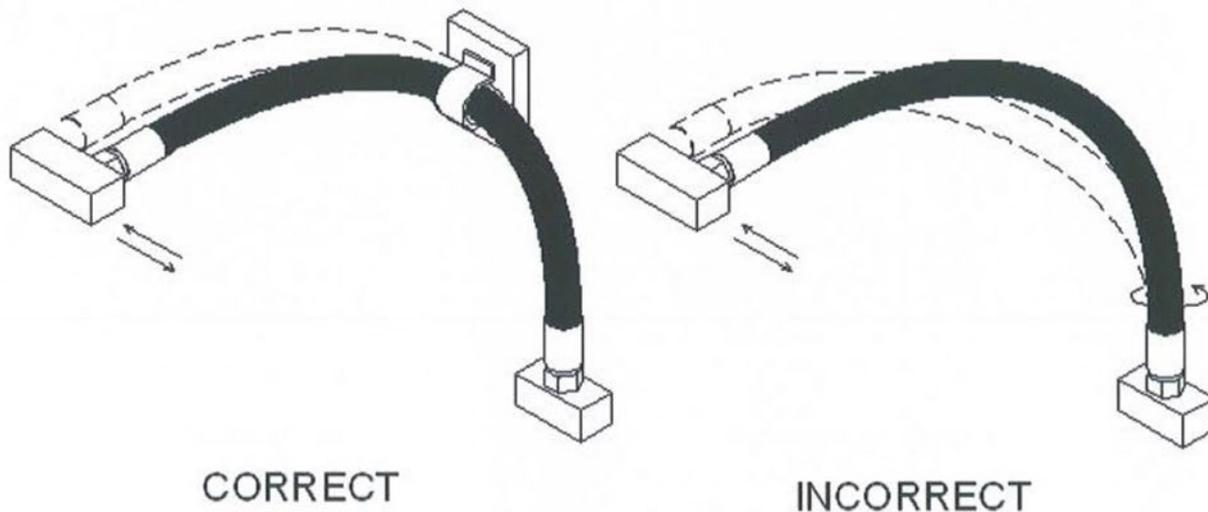
Pressure applied to a twisted hose may shorten the life of the hose or loosen the connections. To avoid twisting, the hose layline or marking can be used as a reference (see Appendix F - Figure 9) if the layline or marking is parallel to the axis of the hose. Twisting can also be avoided by using two wrenches during the installation of swivel connectors.
