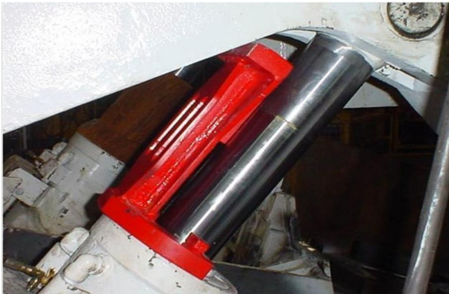
**Note:** Load-locks and other hydraulic componentry for example cylinders can fail. Hence the need for a mechanical stop as shown in the picture above.
