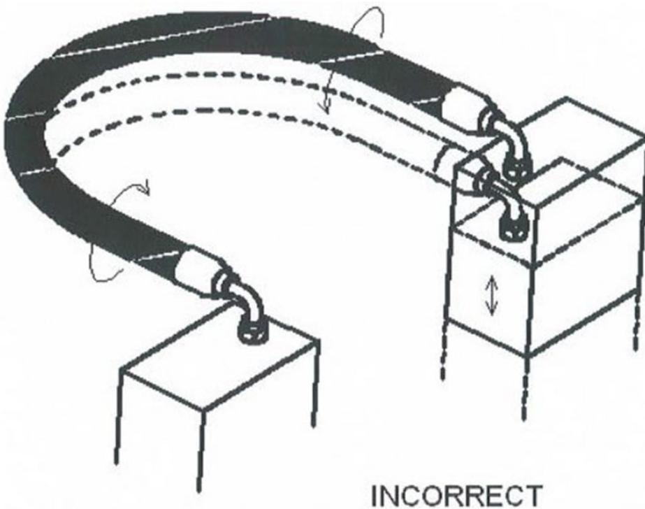
If a hose follows a compound bend, couple it into separate segments or clamp it into segments that each flex in only one plane. See Appendix F - Figure 8.
