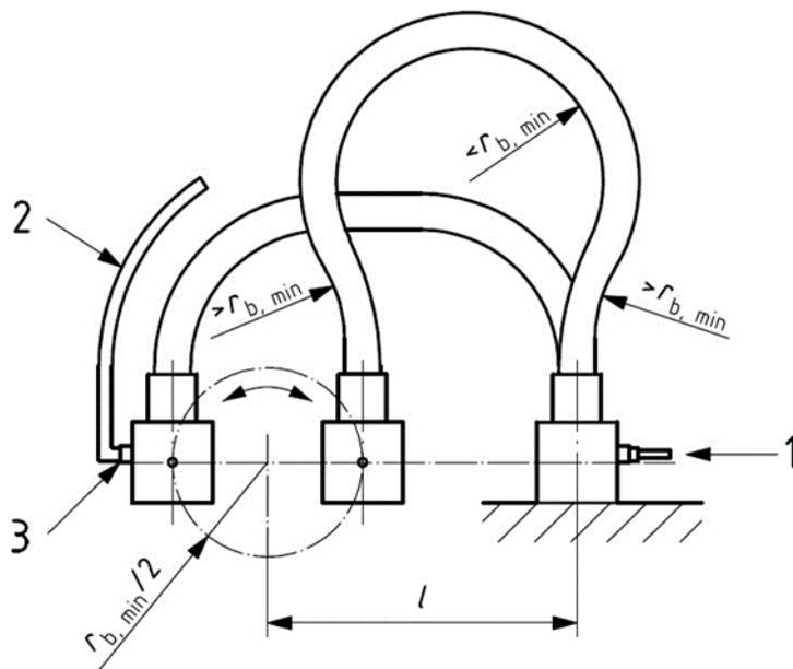
Appendix I- Figure 2 - Hydraulic impulse testing with flexing - Arrangement of test piece using a horizontally reciprocating manifold
