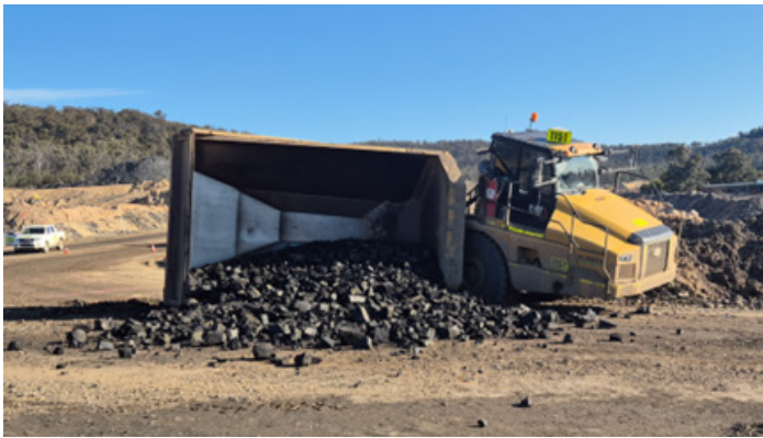
Picture 4. Rolled articulated dump body with spilled material
