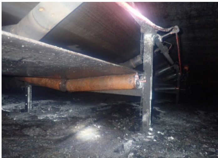
Picture 20. Smoke damage on conveyor structure
