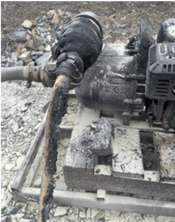
Picture 19. Charred pump after ignition incident
