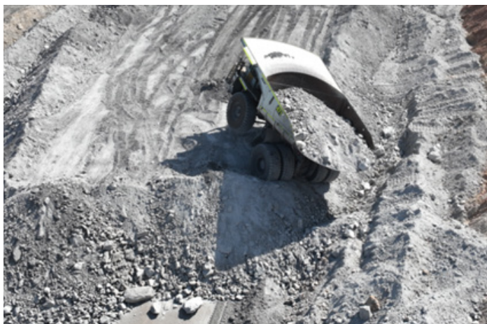
Picture 18. Slumped truck with raised wheel
