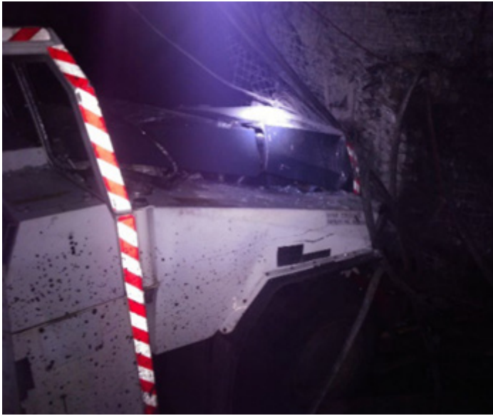
Picture 11. Collision damage at intersection
