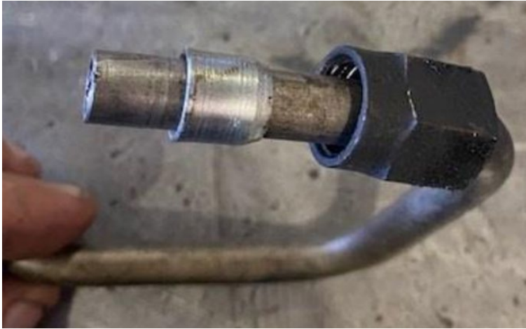
Figure 6: Failed fitting showing no engagement marking on pipe from crush olive
