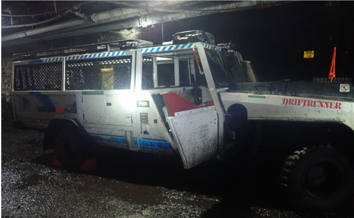
Figure 4: A drift runner lost steering and collided with the rib in a main travel road
