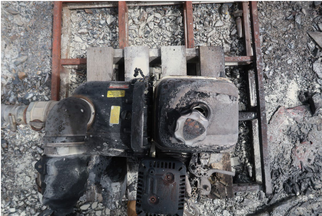
Figure 4: Top view of fire-damaged water pump
