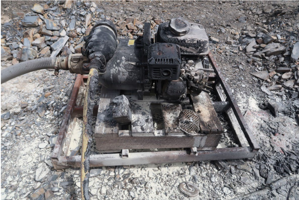
Figure 4: Top view of fire-damaged water pump
