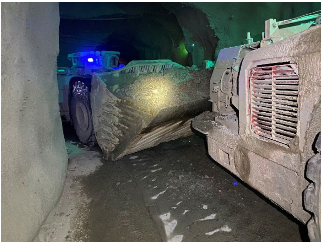
Figure 1: Vehicle collision in an underground metalliferous operation
