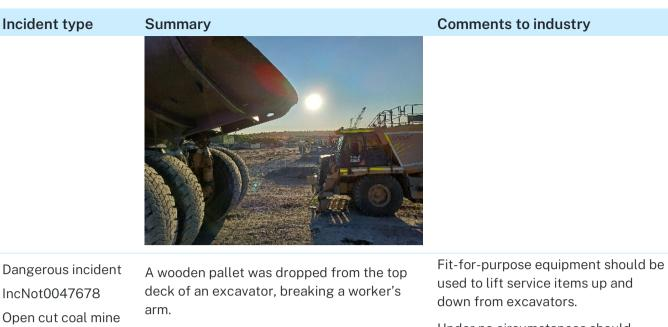
Following a service on the excavator, a worker on the top deck checked the ground area to see if it was clear then dropped a pallet over the guardrail. The pallet weighed 19.12 kg and fell about 7m from the excavator, hitting the worker below on the forearm and hand.
