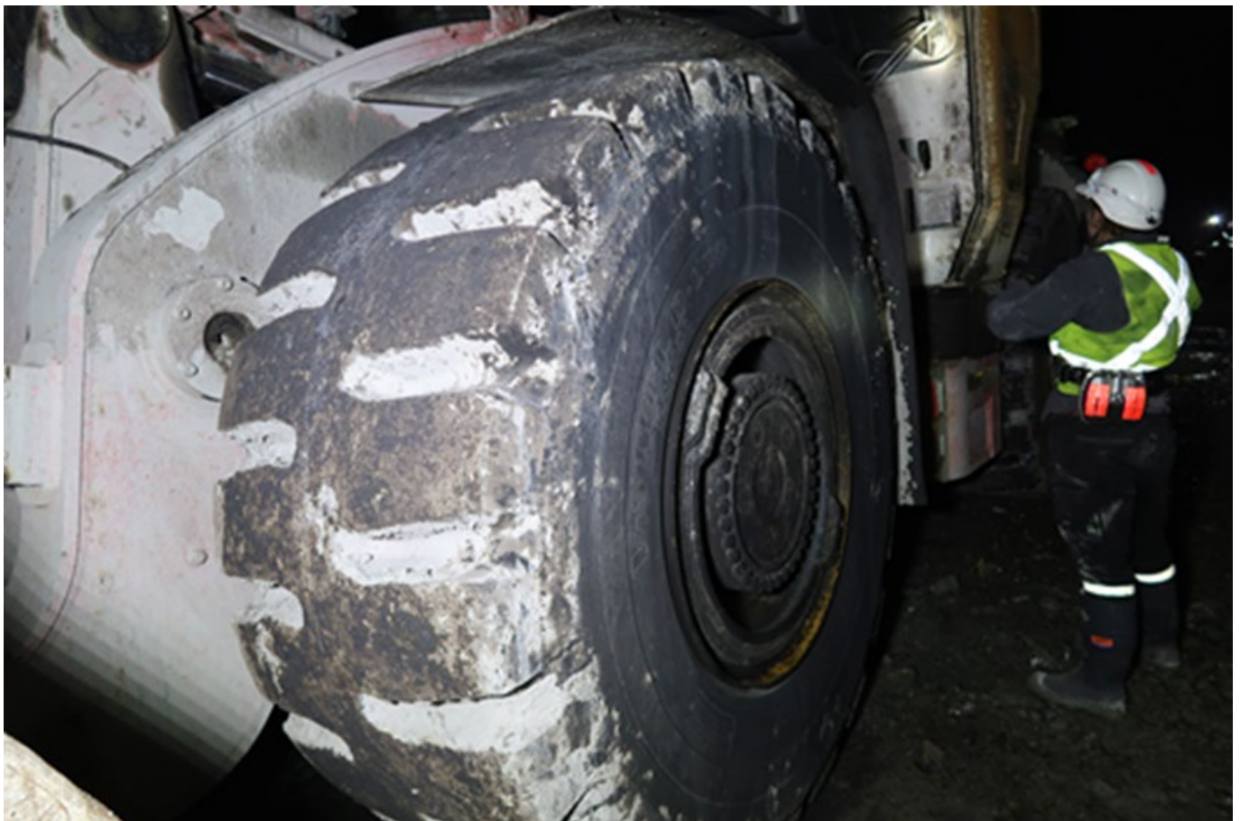
Figure 1: Fire damage to the loader's position one tyre
