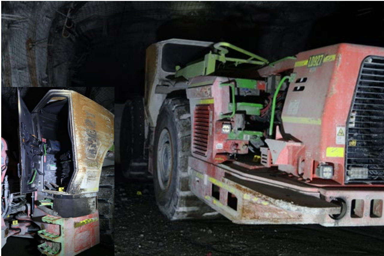
Figure 2: The rear left side of the loader and the operator's cabin with fire damage (inset)
