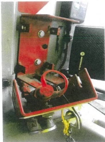
Figure 1 - Actuator panel separated from the mounting bracket
