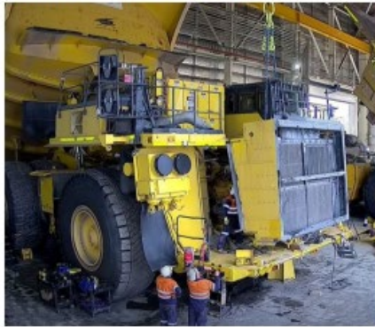
Figure 1: Worker manoeuvring engine module
