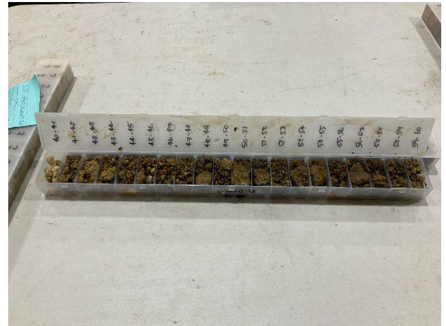
Figure 4 Example of typical chip sample from air core drilling
