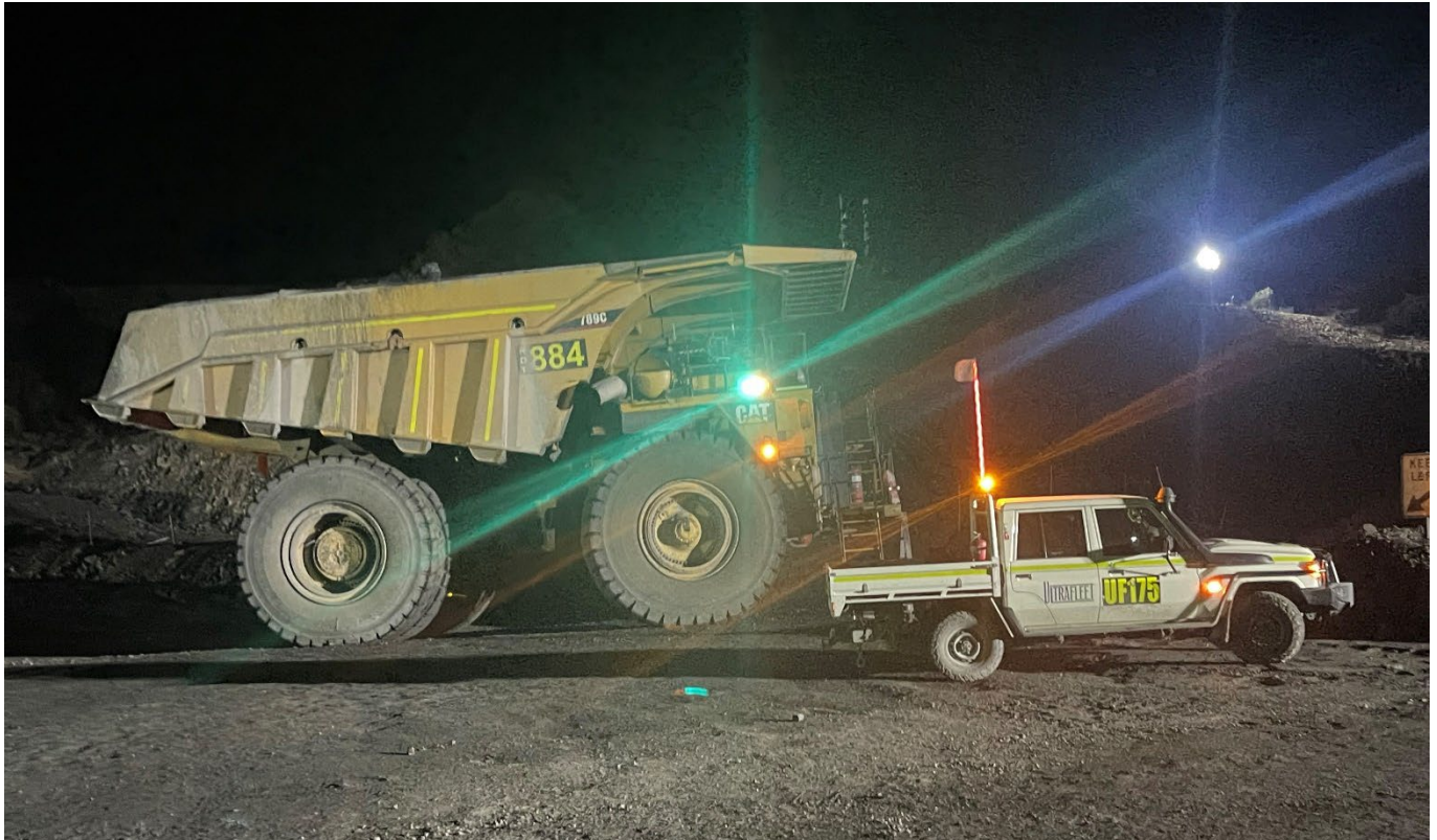
Figure 3: Haul truck and light vehicle near miss incident (vehicle passing haul truck)
